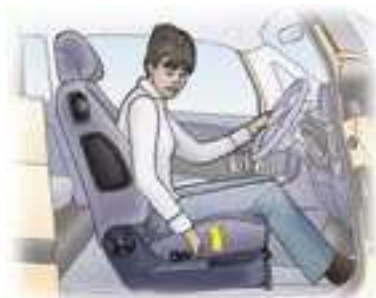
2. Driver's seat height adjustment.
