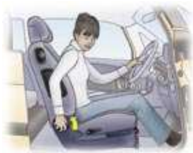
3. Seat back angle adjustment.
