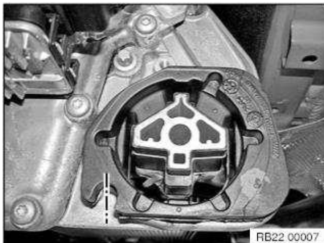
Fig. 11: Observe Installation Position Of Rubber Mount Courtesy of BMW OF NORTH AMERICA, INC.
