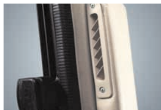
Defroster in the driver's seat Defroster is equipped in the A pillar part of the driver's seat so that the window steam in the inclement weather is removed, thereby for improving the sight of the driver in large scale.
