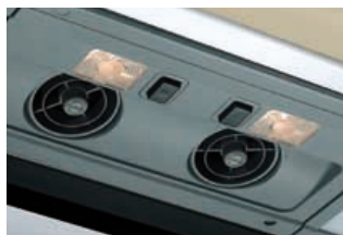
Overhead vent is louvered and adjustable
