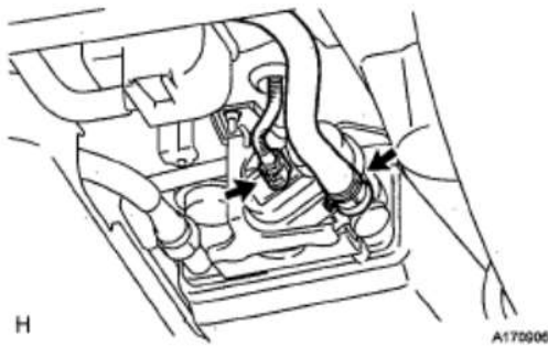
Fig. 12: Locating Hose And Charcoal Canister Connector Courtesy of TOYOTA MOTOR SALES, U.S.A., INC.
