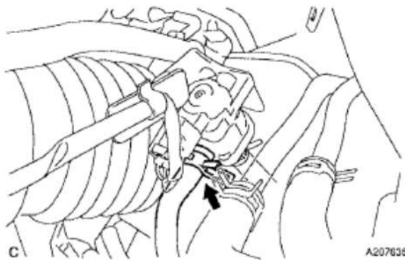
Fig. 6: Locating Vacuum Hose Clip
