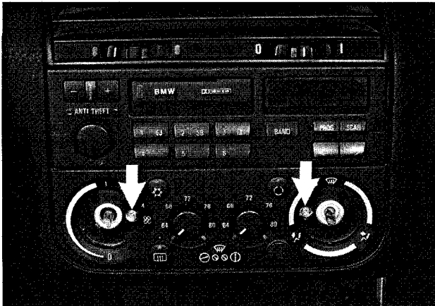
Fig. 22. A/C control head faceplate screws on rotary knob version (arrows). Once screws are removed, faceplate must be unclipped from control head.
