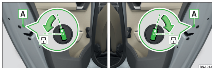
Fig. 194 Emergency locking: Left/right rear door
