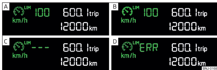
Fig. 142 Segment display: Examples of Speed Limiter status displays
