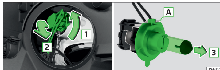
Fig. 210 Changing the bulb for the low beam
