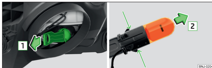
Fig. 212 Changing the bulb for the turn signal light
