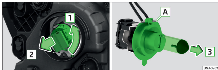
Fig. 211 Changing the bulb for the main beam
