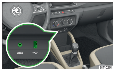
Fig. 89 Installation locations of the AUX and USB inputs
