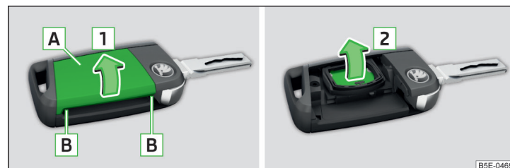
Fig. 192 Remote control key: Remove cover/take out battery
