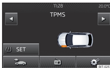
Fig. 148 Button for storing the pressure values/example of the display: the system suggests a change to the front-left tyre pressure
