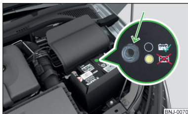
Fig. 172 Vehicle battery: Electrolyte level indicator
