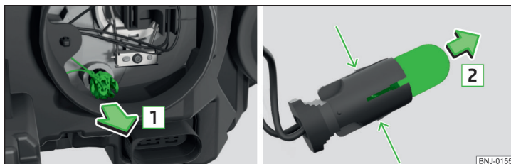
Fig. 208 Change the light bulb for the parking light
