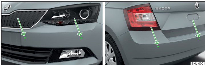
Fig. 133 Installation position of the sensors on the left side of the vehicle: front/rear
