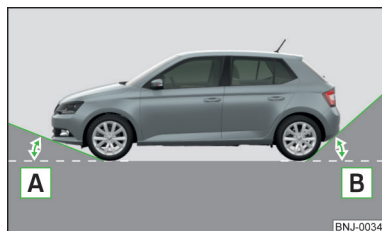
Fig. 220 Principle sketch: Departure angle
