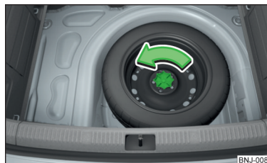
Fig. 180 Taking the wheel out
