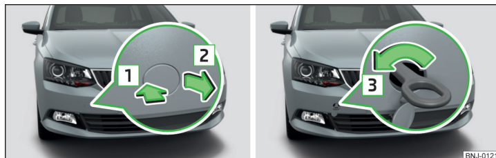
Fig. 190 Removing the cap / installing the towing eye
