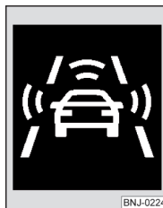
Fig. 146 Symbols in the instrument cluster: Warning or emergency braking at low speed
