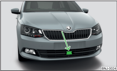
Fig. 144 Mounting location of the radar sensor
