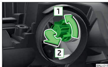
Fig. 207 Changing the bulb for the front turn signal light
