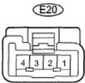
Fig. 5: Identifying E20 Connector Terminal Courtesy of TOYOTA MOTOR SALES, U.S.A., INC.
