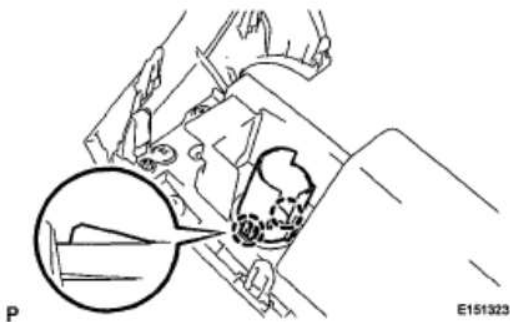
Fig. 50: Identifying Power Outlet Socket Cover Claws Courtesy of TOYOTA MOTOR SALES, U.S.A., INC.
