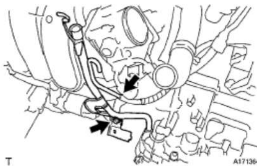
Fig. 31: Locating Transmission Oil Level Gauge Sub-Assembly With Bolt
