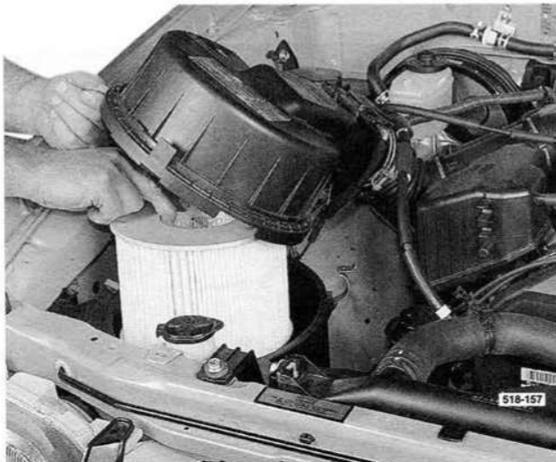
A blocked or restricted air cleaner element can reduce the engine power and increase fuel consumption.
