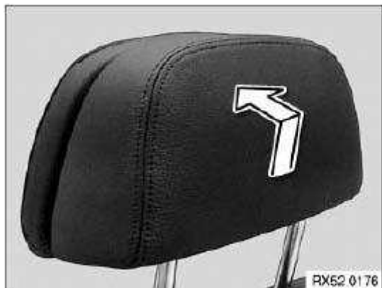
Fig. 23: Clipping Cover Onto Carrier Section Courtesy of BMW OF NORTH AMERICA, INC.
