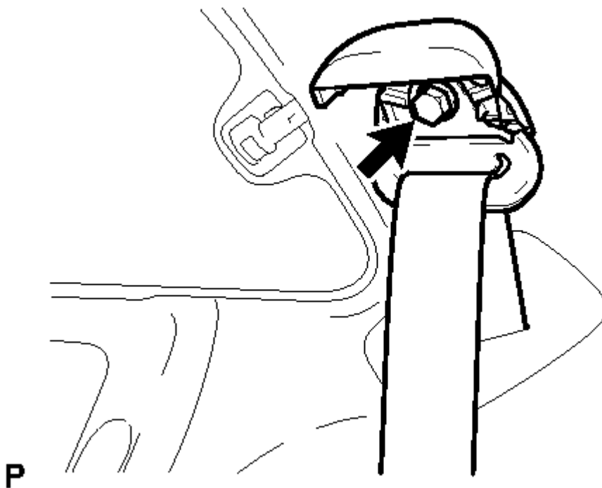
Fig. 143: Identifying Shoulder Anchor & Fastener Courtesy of TOYOTA MOTOR SALES, U.S.A., INC.
