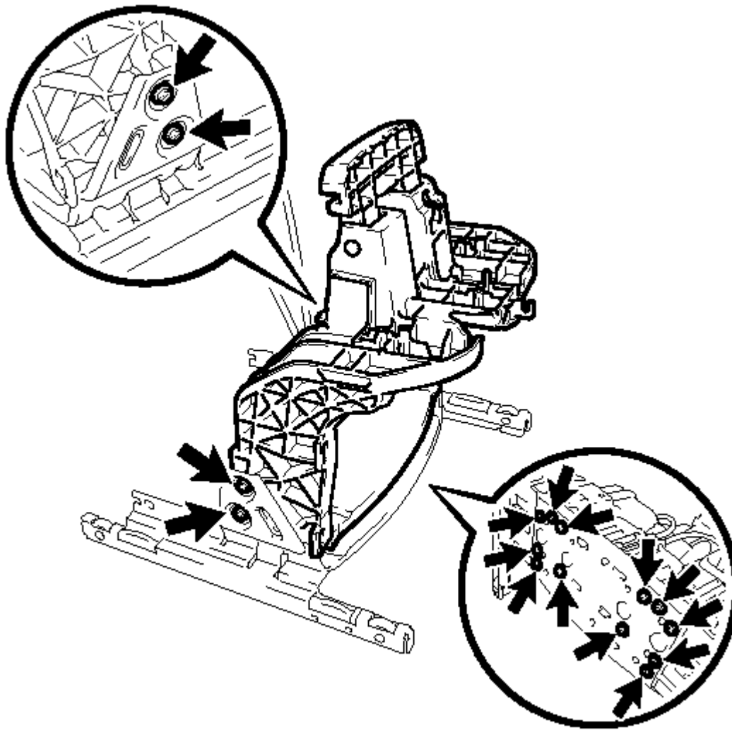
Fig. 82: Identifying Console Compartment Door Hinge Sub-Assembly & Fasteners Courtesy of TOYOTA MOTOR SALES, U.S.A., INC.
