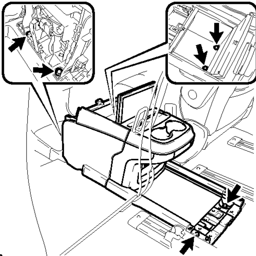
Fig. 66: Identifying Console Assembly & Fasteners Courtesy of TOYOTA MOTOR SALES, U.S.A., INC.
