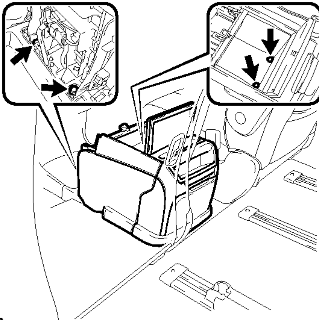
Fig. 98: Identifying Console Assembly & Fasteners Courtesy of TOYOTA MOTOR SALES, U.S.A., INC.
