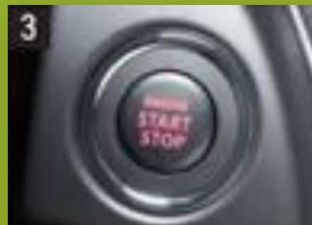
3 Hold the clutch pedal down (or brake on CVT) then press the engine-start button
