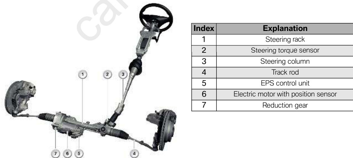
Electric power steering with parallel-mounted motor
