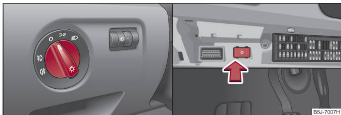
Fig. 36 Dash panel: Light switch / fuse box: Switch for daylight driving lights
