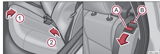
Fig. 53 Fold the seat cushion forwards / unlock the seat backrest
