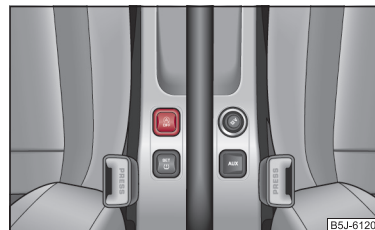
Fig. 99 Centre console: Button for the START-STOP system
