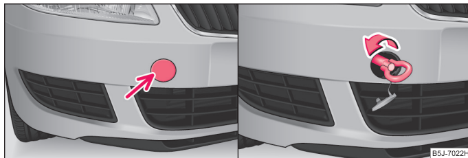
Fig. 159 Front bumper: Cover / installing the towing eye
