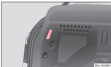
Fig. 177 Remove the luggage compartment light
