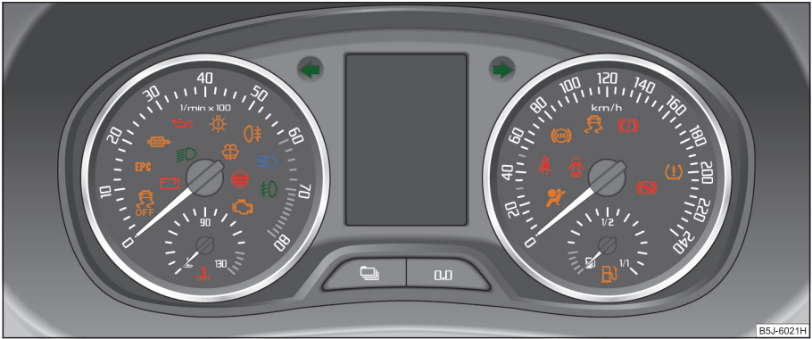
Fig. 22 Instrument cluster with warning lights
