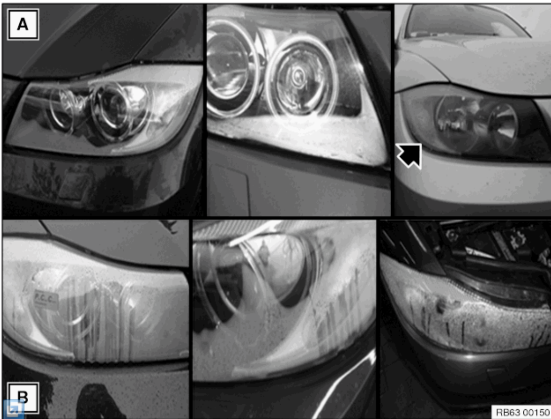
Fig. 16: Identifying Permissible And Impermissible Fogging Courtesy of BMW OF NORTH AMERICA, INC.
