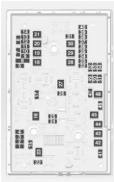
Vauxhall Cascada – fuse box – engine compartment
