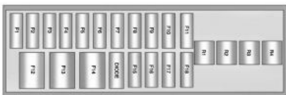
Cadillac ELR – fuse box – instrument panel (left side)
