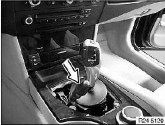
Fig. 74: Releasing Transmission Lock
