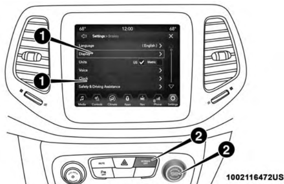
Uconnect 4C/4C NAV With 8.4-inch Display Buttons On The Touchscreen And Buttons On The Faceplate
