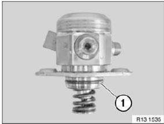
Fig. 4: Replacing Sealing Ring
