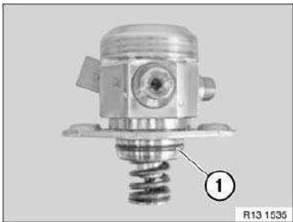
Fig. 8: Identifying Sealing Ring Courtesy of BMW OF NORTH AMERICA, INC.
