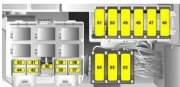
Vauxhall Combo C – fuse box – engine
