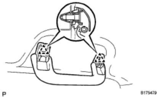
Fig. 31: Identifying Assist Grip Springs
