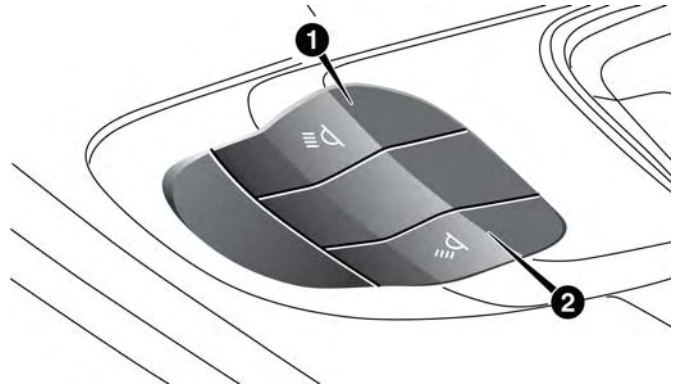
Courtesy Light Switches
