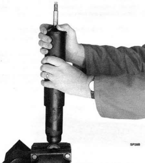
Checking for defective shock absorber operation.
