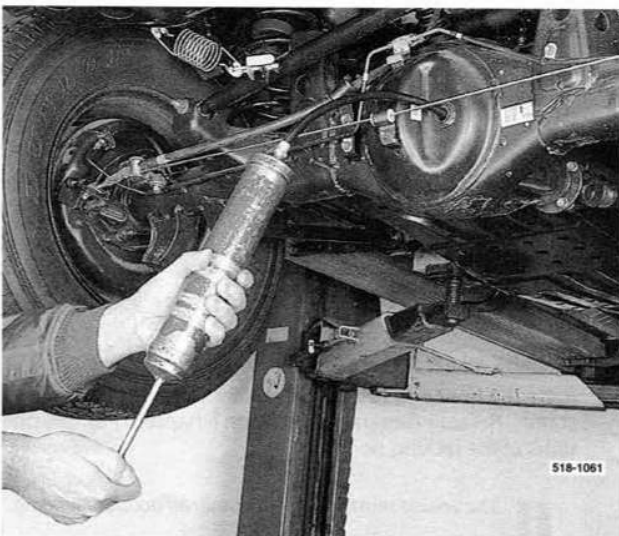
Filling the rear axle with an oil gun.
