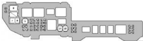
Lexus ES300 – fuse box – engine compartment
