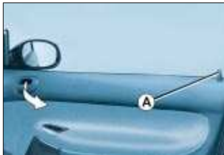
Opening the doors from inside
