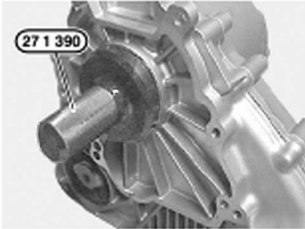
Fig. 3: Driving In Radial Shaft Seal (NV125 Transmission Shown) Courtesy of BMW OF NORTH AMERICA, INC.
