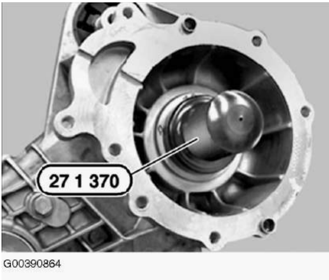
Fig. 8: Driving In Radial Shaft Seal (LWX-500) Courtesy of BMW OF NORTH AMERICA, INC.
