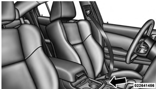
Inserting Latch Plate Into Buckle
