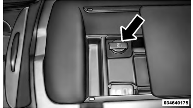
Center Console Power Outlet
