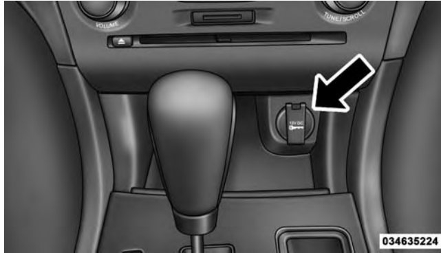
Front Power Outlet
