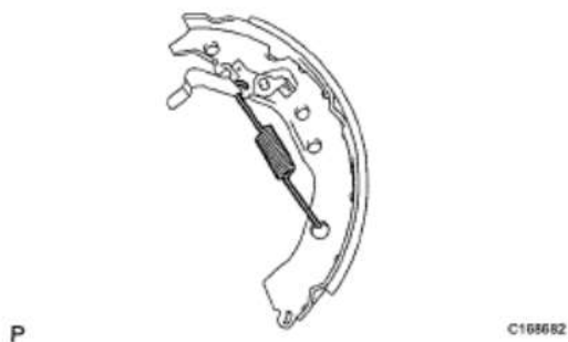
Fig. 121: Identifying Automatic Adjust Lever Tension Spring Courtesy of TOYOTA MOTOR SALES, U.S.A., INC.
