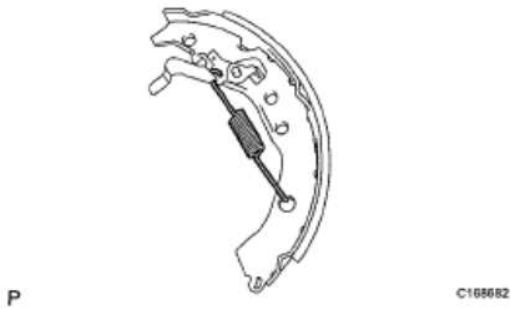
Fig. 109: Identifying Automatic Adjust Lever Tension Spring Courtesy of TOYOTA MOTOR SALES, U.S.A., INC.
