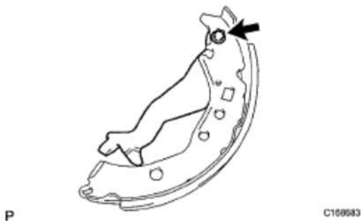
Fig. 110: Locating Parking Brake Shoe Lever Courtesy of TOYOTA MOTOR SALES, U.S.A., INC.
