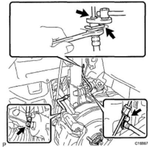
Fig. 98: Removing Front Brake Flexible Hose Courtesy of TOYOTA MOTOR SALES, U.S.A., INC.
