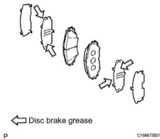
Fig. 93: Identifying Disc Brake Grease Applying Area Courtesy of TOYOTA MOTOR SALES, U.S.A., INC.
