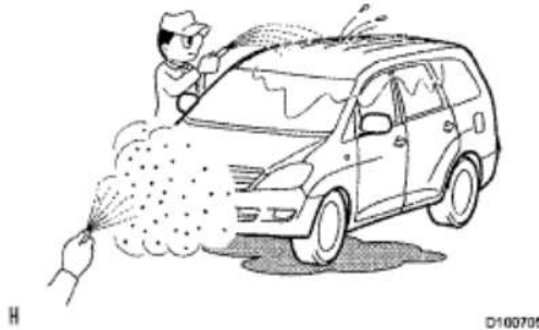
Fig. 30: Identifying Water Sprinkling Method
