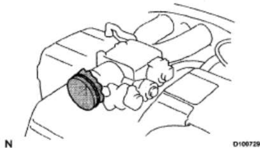
Fig. 20: Covering Openings Of Removed Parts And Engine Openings Courtesy of TOYOTA MOTOR SALES, U.S.A., INC.
