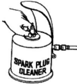
Fig. 11: Cleaning Spark Plugs
