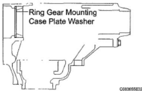
Fig. 79: Identifying Ring Gear Mounting Case Plate Washer Location Courtesy of TOYOTA MOTOR SALES, U.S.A., INC.
