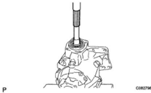
Fig. 51: Identifying Driven Pinion, Transfer Driven Pinion Rear Bearing Inner Race And Transfer Pinion Bearing Spacer
