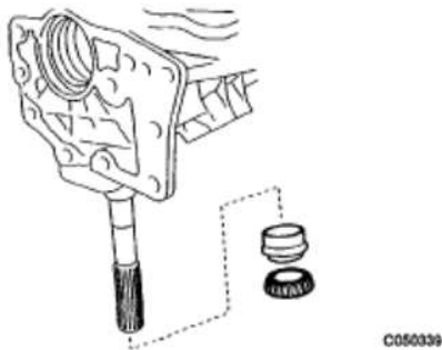
Fig. 65: Identifying Transfer Pinion Bearing Spacer And Inner Race To Driven Pinion Courtesy of TOYOTA MOTOR SALES, U.S.A., INC.
