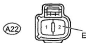
Fig. 6: Identifying A22 Washer Fluid Level Warning Switch Connector Courtesy of TOYOTA MOTOR SALES, U.S.A., INC.
