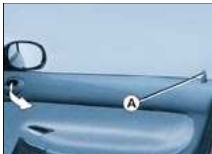
Opening the doors from inside
