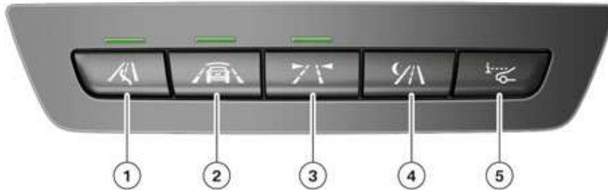
F01/F02 LCI driver assistance system operating facility
