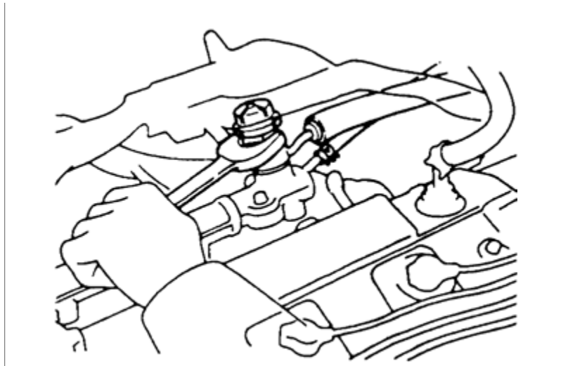
Fig. 2: Unbolt and remove the fuel delivery pipe and injectors as an assembly
