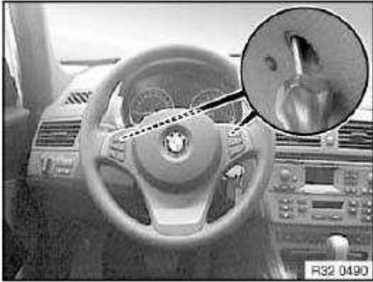
Fig. 82: Inserting Torx Screwdriver (T30) Horizontally Into Opening On Reverse Side Of Steering Wheel Courtesy of BMW OF NORTH AMERICA, INC.
