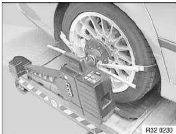
Fig. 16: Attaching Quick-Clamping Holder/Quick-Clamping
