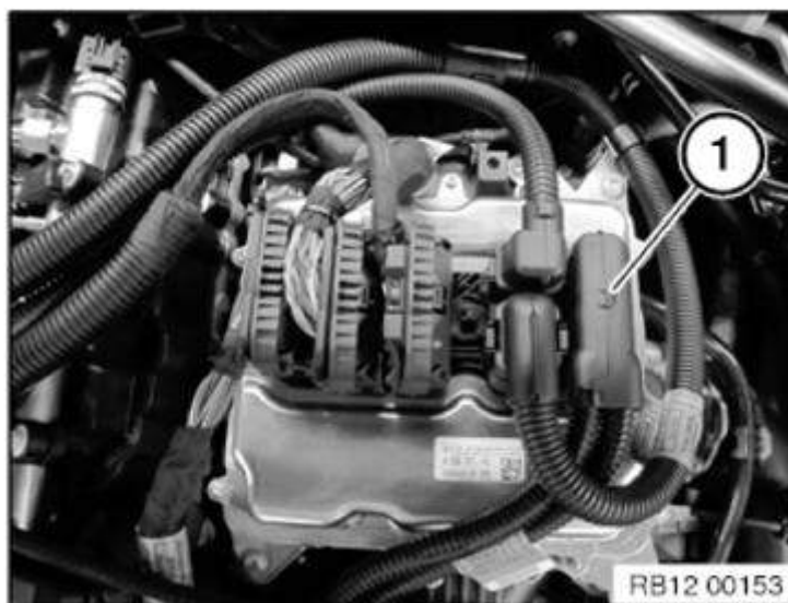
Fig. 159: Identifying Connector From Control Unit Courtesy of BMW OF NORTH AMERICA, INC.
