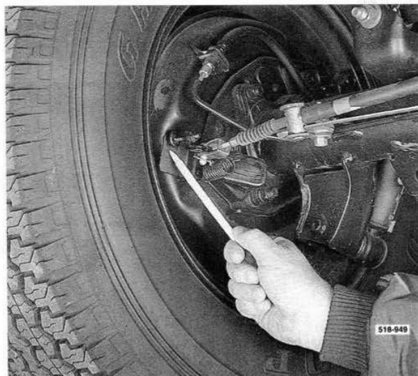
Turn the adjusting screw until it touches the backing plate, then back off one turn.
