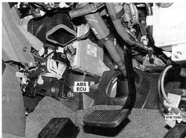
Location of the ABS electronic control unit (ECU).
