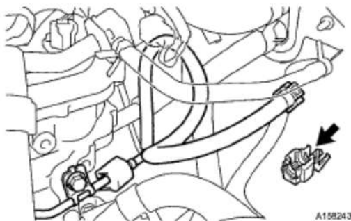
Fig. 46: Locating Fuel Pipe Clamp Courtesy of TOYOTA MOTOR SALES, U.S.A., INC.
