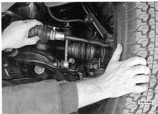
Checking the tie rod ball housing for wear by moving the wheel and feeling movement at the ball.
