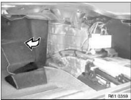
Fig. 55: Removing Front Side Trim Panel Courtesy of BMW OF NORTH AMERICA, INC.
