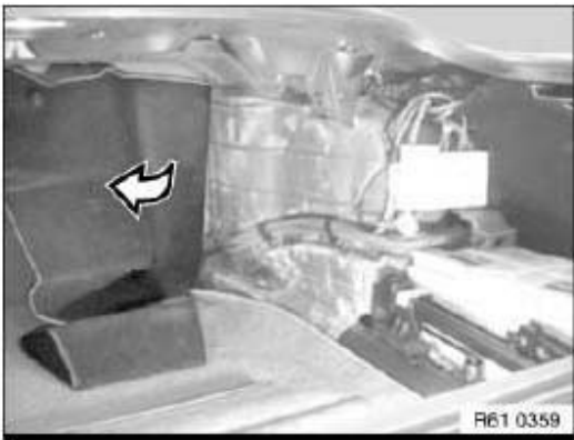
Fig. 55: Removing Front Side Trim Panel Partly Courtesy of BMW OF NORTH AMERICA, INC.
