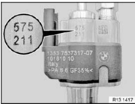
Fig. 28: Identifying Adjustment Value Printed In Blocks Of Digits On Injector Courtesy of BMW OF NORTH AMERICA, INC.
