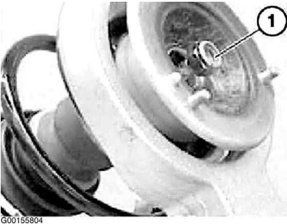
Fig. 24: Locating Self-Locking Nut On Piston Rod Courtesy of BMW OF NORTH AMERICA, INC.
