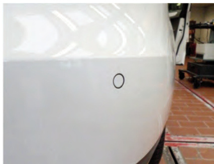
Ultrasonic sensor in the rear end 9_51_13
