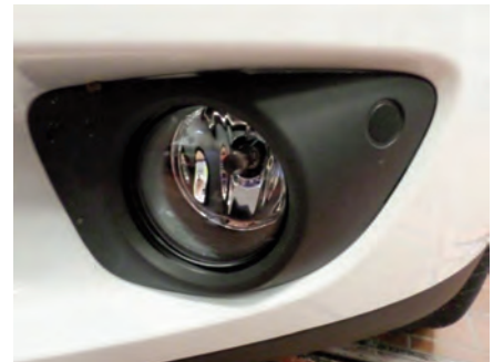
Ultrasonic sensor in the front apron 9_50_13
