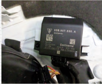
Gateway CU, under rear seat
