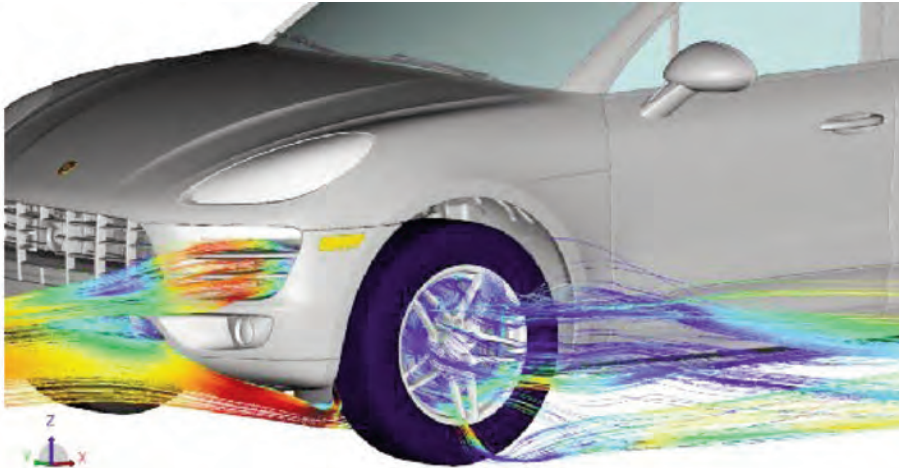
Air flow for brake cooling
