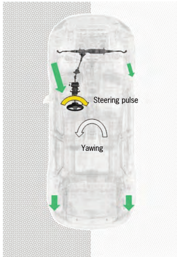
Steering recommendation for \mu -split braking
