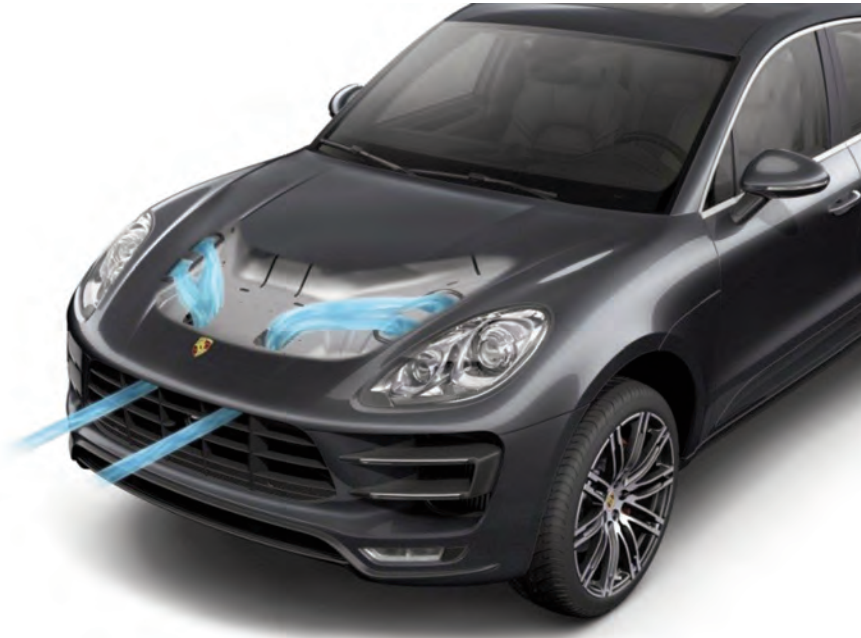
Intake opening through the hood
