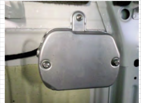
PVTS control unit, under rear seat bench
