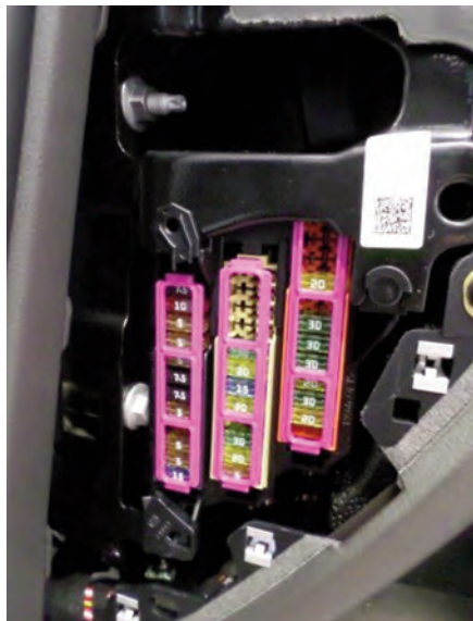
Fuse carrier, Driver's side
