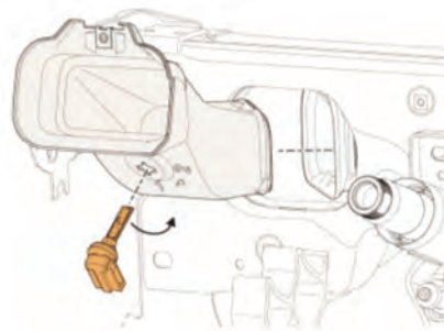
Temperature sensor for passenger air vent (left)
