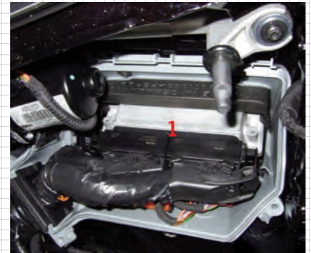
DME control unit in E-box
