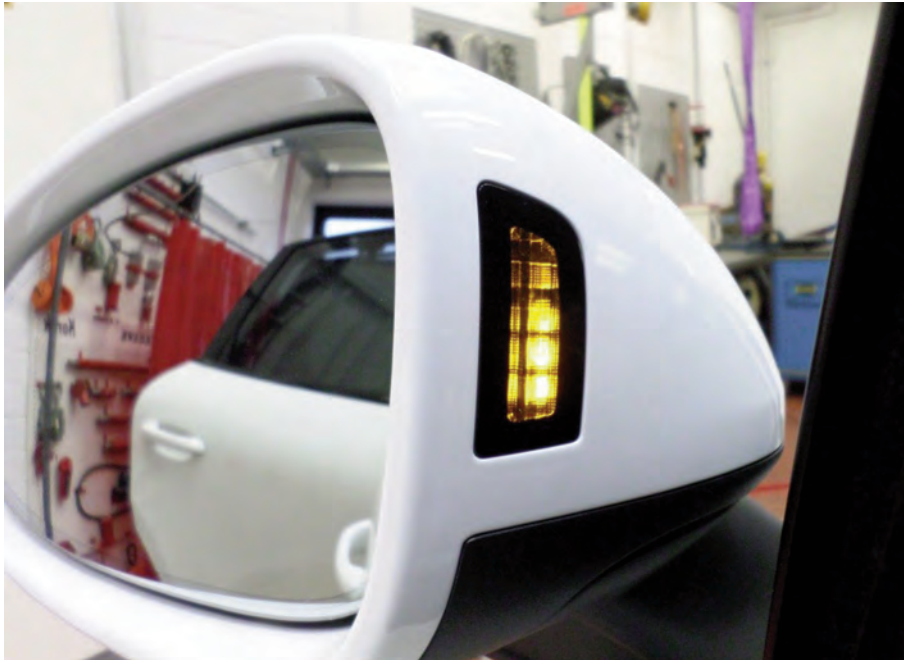
Readiness indicator LEDs in the exterior mirrors
