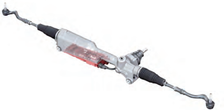
Steering gear (tie rods shown without air-guide vanes)
