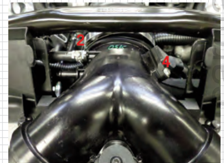
Installation position of booster pressure sensor
