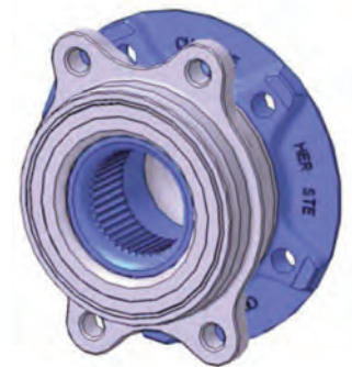
Wheel bearing (wheel carrier side) 4_32_13
