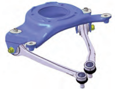
Mounting saddle with control arms fitted
