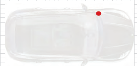
Installation position of front-end electronics control unit
