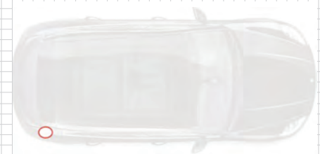
Installation position of rear-end electronics control unit
