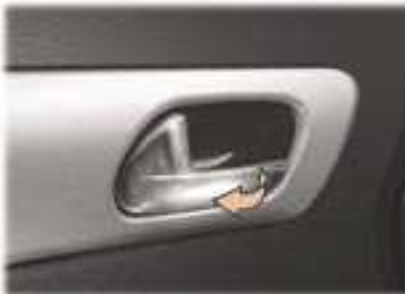
Opening the doors from inside
