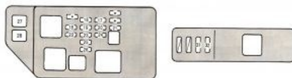
Lexus ES – fuse box – engine compartment
