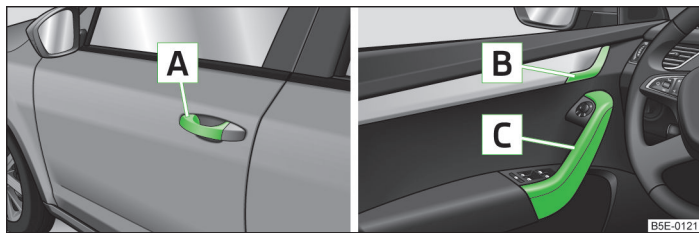
Fig. 17 Door handle/door opening lever: outside/inside
