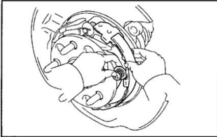
Fig. 7: Rear Disc Brake Parking Brake Removal Procedure (2 Of 2)
