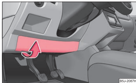
Fig. 204 Bottom side of the dash panel: fuse cover
