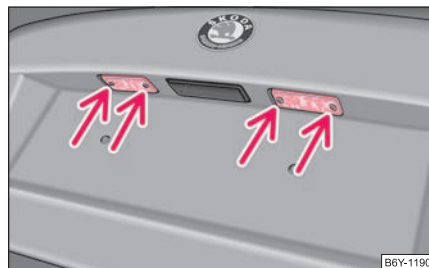
Fig. 216 Remove the licence plate light
