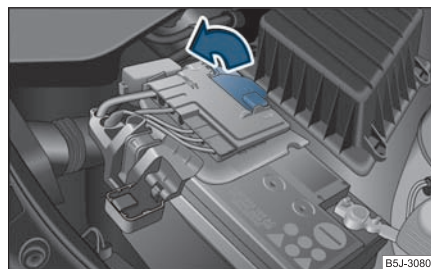
Fig. 187 The battery: pull up the cover (manual gearbox)
