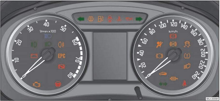
Fig. 30 Instrument cluster with warning lights
