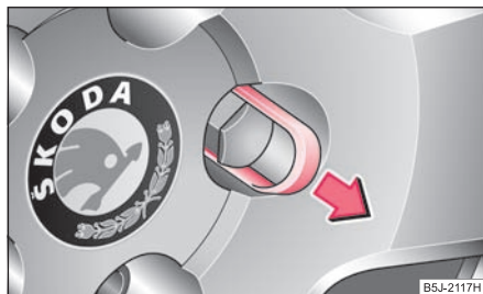
Fig. 196 Changing a wheel: Pull off cap from the wheel bolt
