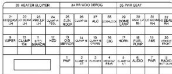
Cadillac Catera – fuse box – instrument panel
